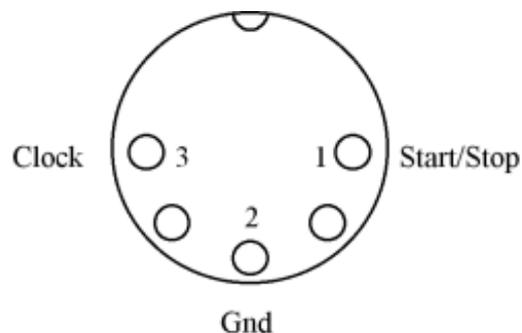
In some applications the remaining pins (4 and 5) are even used as "tap", "fill in" or "reset and start". But this differs from device to device.
